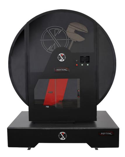
The Hoytom pendulum impact tester has been designed to test metals according to the Charpy or Izod impact testing standards. It is available in capacities from 150 to 750 Joules.
