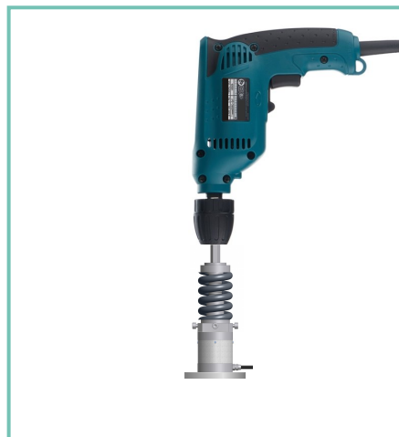
Torque measurement using fidaptor
