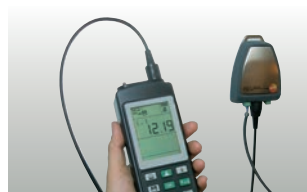
Inspection of transmitters with 4 to 20 mA interface
