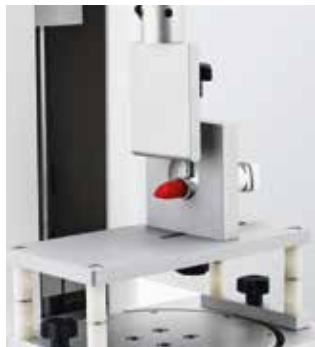
TX-LCF : LIPSTICK CANTILEVER FIXTURE (Ref. 130147R) Accessory to measure strength of lipstick.
