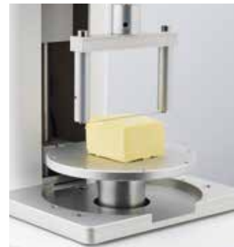
TX-WSF : WIRE SHEAR FIXTURE (Ref. 130076R) Accessory to measure consistency of product as Butter or Cheese.
