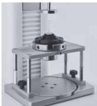
TX-SAF : SYRINGE ACTUATOR FIXTURE (Ref. 130145) Study of needed strength to use syringe.
