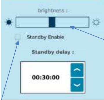
Choose if you want to switch off automatically your device after no using. After selecting "Standby enable", you will have to set time. Your device will be switch off after this time.
