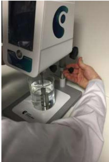
Wait until the temperature of the sample is within the prescribed limits (if you have temperature probe with your device).
