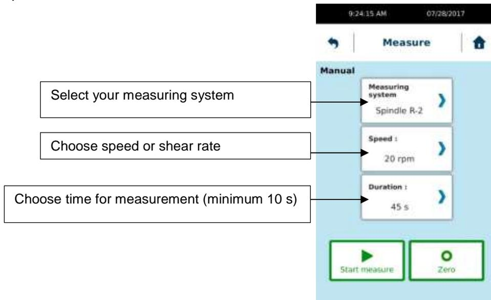
**Rq** : If « Time » = 0, you could modify « speed » during the measurement. This could help you to define the best conditions to work on your sample.
