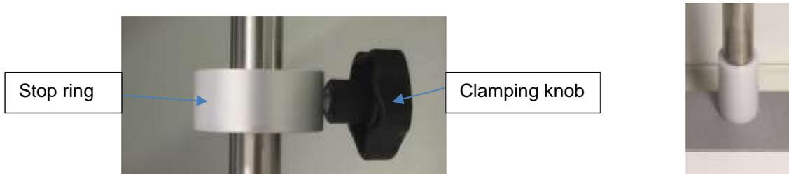
The rod is equipped with a white Teflon ring acting as a stop, thus avoiding the arm being in a position that is too low.
