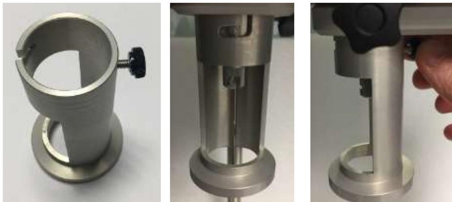
The screw locks the centring piece on the base of the viscometer.
