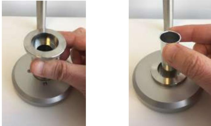
Use handle and screw of arm (see section 1.2) to gently lower the measuring head. The centring piece must completely cover the edge of the disposable cup holder.
