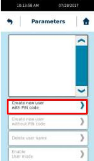
The diagram shows the transition from the 'Parameters' menu to the 'User name' sub-menu. In the 'User name' sub-menu, four options are listed: 'Create new user with PIN code', 'Create new user without PIN code', 'Delete user name', and 'Enable User mode'. The first option is highlighted in red. A blue arrow points from the 'User name' option in the first screenshot to the 'Create new user with PIN code' option in the second screenshot.
