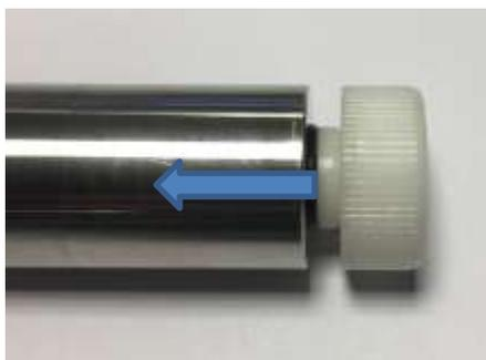
The first insertion of the cap can be difficult. You must use some silicone grease to facilitate installation.
