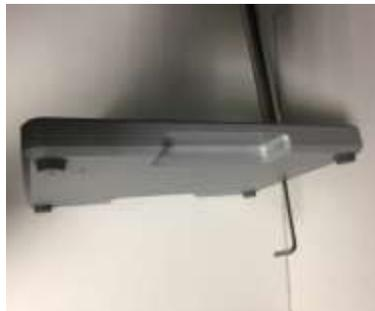
Then make sure to insert the white Delrin cylinder and set it to the lowest position. Then place the stop ring on the stainless steel rod. Then place arm on rod, respecting the direction as described below. The arm is equipped with two buttons and a handle. You can change them for your convenience if you are left-handed.
