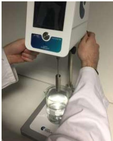
Adjust the position of the viscometer in the sample to immerge the mobile to the predefined mark (the lowest for discs # 2 -6, the highest for disc # 1), so as to immerge the Pt100 probe at least 3 mm (only for models equipped with a temperature probe integrated into the measuring head. If an external temperature sensor is used, the liquid level must always be in
