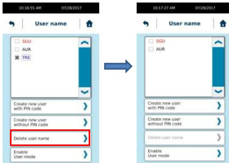
To use the operator accounts you must activate the mode. Device will ask you to select user name you want to use. By returning to the Main Menu, you will see the name of the operator in use. By clicking on the arrow below the name of the operator, you can switch off the B-ONE or change operator.
