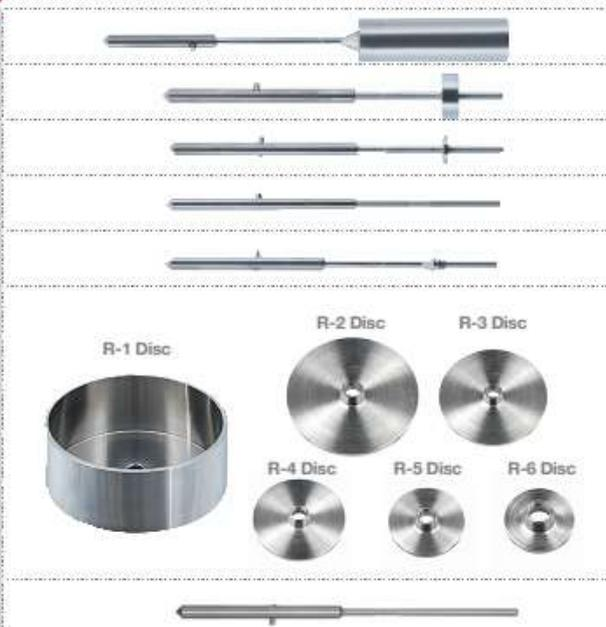
These spindle are composed of two groups. The mobiles L are intended for low viscosity fluids and R mobiles for medium to high viscosities (see tables below):
