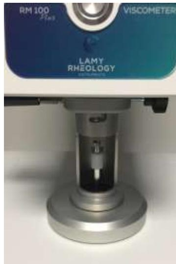
When the measuring head is properly positioned, there is no need to lock the position using the screw on the arm. Also, be sure to allow sufficient time for stabilization if the measurement temperature is different from the room temperature (at least 10 minutes) before taking your measurement.
