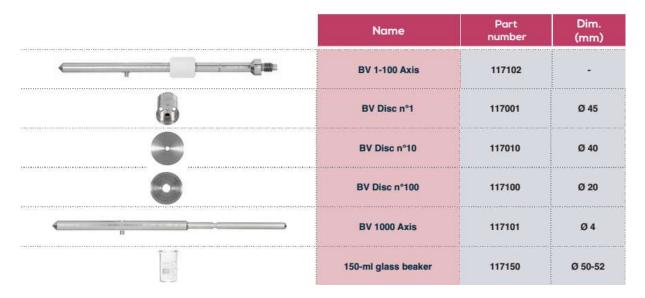
This spindle allow measurement of huge viscosity range as showing below.
