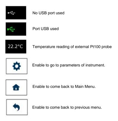
Some B-ONE PLUS are equipped with an external temperature sensor. When it has been ordered, the temperature display is shown at the top right of the screen. If this is not the case, see section 2.2.5.9 to enable reading. The USB port icon indicates that a USB flash drive has been connected. This is only used to update the firmware and cannot be used to transfer the results.
