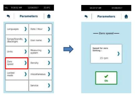
You have to use the same speed as for your viscosity measurement. Then zero setting is finished, you have to click "Ok" to validate it.
