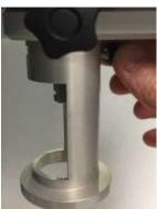
The screw locks the centring piece on the base of the viscometer.
