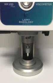
When the measuring head is properly positioned, there is no need to lock the position using the screw on the arm. Also, be sure to allow sufficient time for stabilization if the measurement temperature is different from the room temperature (at least 10 minutes) before taking your measurement.
