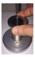
Use handle and screw of arm (see section 1.2) to gently lower the measuring head. The centring piece must completely cover the edge of the disposable cup insert.
