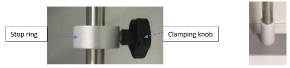
The rod is equipped with a white Teflon ring acting as a stop, thus avoiding the arm being in a position that is too low.
