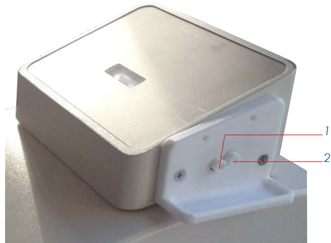
Fig. hose connections on the frequency oscillator
