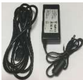
Cable and power supply for measuring head
