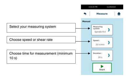
$\mathbf{Rq}$ : If « Time » = 0, you could modify « speed » <u>during</u> the measurement. This could help you to define the best conditions to work on your sample.
