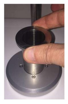
Use the arm handle and screw (see section 1.2) to gently lower the measuring head. The centring piece must completely cover the rim of the tube.
