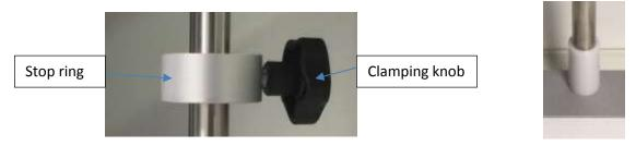
The rod is equipped with a white Delrin ring acting as a stop, thus avoiding the arm being in a position that is too low.
