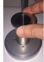
Use handle and screw of arm (see section 1.2) to gently lower the measuring head. The centring piece must completely cover the edge of the disposable cup insert.
