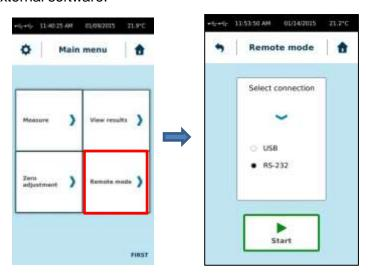
**Rq**: With mini USB connection, respect strictly the order to start, and if any communication is possible re-connect the USB cable on computer and wait it is recognized before start the communication.
