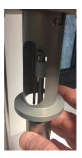
You must then install the MK-DIN cylinder on the viscometer axis as shown in the photo above.
