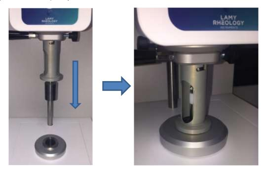
When the measuring head is properly positioned, there is no need to lock the position using the screw on the arm. Also, be sure to allow sufficient time for stabilization if the measurement temperature is different from the ambient temperature (at least 10 minutes) before making your measurement.
