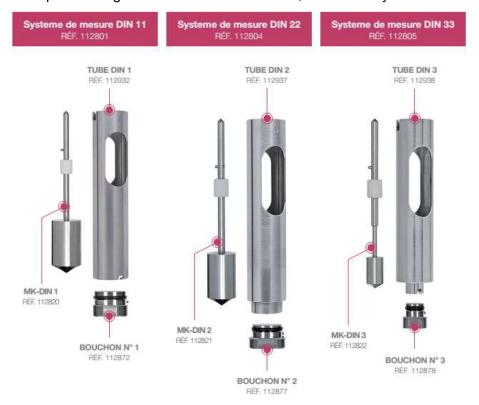
In addition to these measuring systems, a DIN X tube with a MK-DIN X+1 cylinder can be used. Thus, MS DIN 12, MS DIN 13 and MS DIN 23 measuring systems can also be used. The first digit always indicates the number of the tube and the second digit the number of the cylinder MK. There is also a measuring system MS DIN 19 which uses the DIN tube 1 and MK-DIN 9 cylinder.
