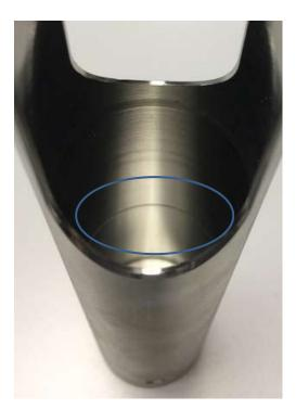
You must then install the MK-DIN cylinder on the viscometer shaft as shown in the photos below.
