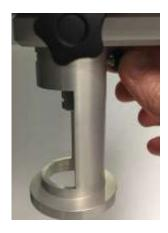
The screw locks the centring piece on the base of the viscometer.
