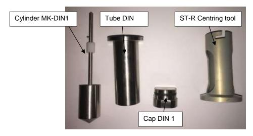
The first step is to install the cap on the tube as shown in the photo below. Also check that the gasket is properly installed on the cap.
