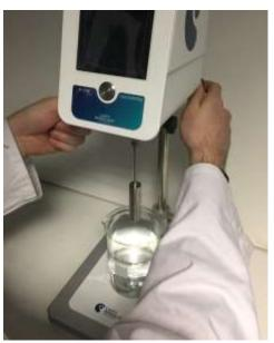
Adjust the position of the viscometer in the sample to immerge the mobile to the predefined mark (the lowest for discs # 2 -6, the highest for disc # 1), so as to immerge the Pt100 probe at least 3 mm (only for models equipped with a temperature probe integrated into the measuring head. If an external temperature sensor is used, the liquid level must always be in the mark on the axis mobile). Be careful that the tip of the mobile is 10 mm or more from the bottom of the beaker.
