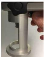
The screw locks the centring piece on the base of the viscometer.
