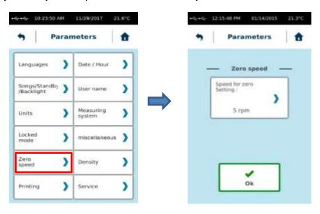
You have to use the same speed as for your viscosity measurement. Then zero setting is finished, you have to click "Ok" to validate it.
