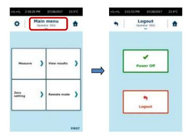
If the instrument is switched off while operator mode is activated, device will ask you to select the operator you want use then device will be switched ON.
