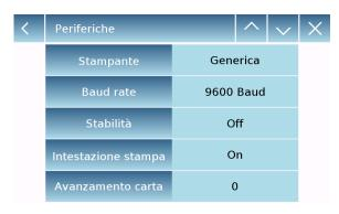
In the "**Peripherals**" menu screen, the values of the parameters set can be immediately verified (in the box to the right of the parameter).
