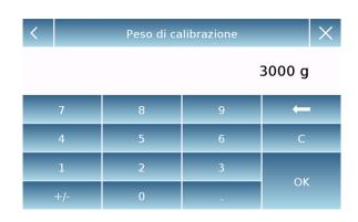
After selecting the "select mode", touch the Weight setting key to set the desired weight value.
