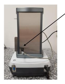
Connect the temperature probe to the device.
