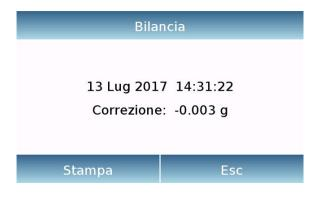
Calibration data: in the calibration data screen, you can check the date on which the last calibration was carried out, the way it was carried out, the value of the weight used and the correction made with respect to the previous calibration. Touching the "Print" key you can print the displayed data.
