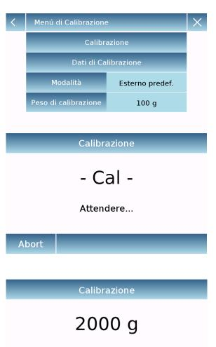
In the calibration menu, you can carry out the calibration, view and print the data relating to the last calibration and set the calibration mode.
