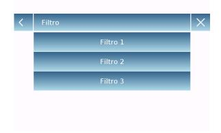
Filter: the filter function allows speeding up or slowing down the response of the scale according to the weighing requirements and environmental conditions. By selecting level 1, the response will be immediate but the scale will remain more sensitive to environmental disturbances such as ventilation and vibrations. As the level increases, the response will be slower and the indication more stable
