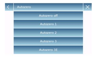
• Autozero: the automatic zero correction constantly adjusts the zero value. These possible variations may be due, for example, to the dirt that can be deposited on the plate. You can deactivate this function by selecting the "Off" mode. Level 1 is the one with the least correction up to level 3E that is the maximum correction.
