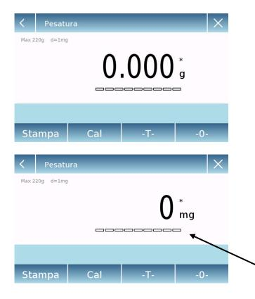
In the central part of the weighing screen, the weight detected by the device is displayed. The weight is expressed in grams. By touching the unit of measurement symbol, you can switch from displaying the weight from grams "g" to milligrams "mg" and vice versa
