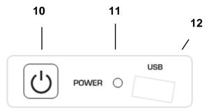
After connecting the power supply to the mains, the device will start automatically without having to press the power button.
