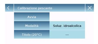
If the mode with known solution is selected. touch the "Titre (20°C)" key and enter the value of the solution at a temperature of 20°C.
