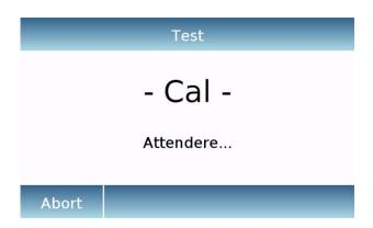
After confirming with the "Start" key, the scale calibration will be performed automatically.
