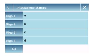
In the print header screen, touch the rectangles indicating the line number to automatically activate the alphanumeric keyboard and enter the desired text with a maximum number of 40 characters per line.
