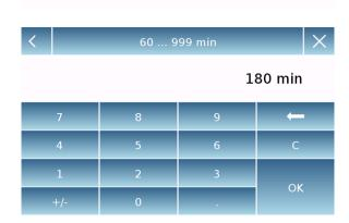
To change the autocalibration interval, touch the "Calibration interval" key and set the desired range that must be between 60 and 999 minutes.
