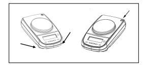
**Wait** 30 minutes after switching on and calibrate the device after leveling it. For the calibration procedures, refer to the "**Device calibration chapter**". Perform calibration of the device whenever it is moved to another place.
