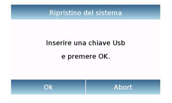
Insert the flash drive into the USB port located on the left side of the device, and press the "OK" key.
