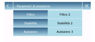
In the "Weighing parameters" screen, the set values can be checked immediately (in the box to the right of the parameter).
