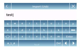
If the USB key has been inserted correctly, after confirmation, the alphanumeric keyboard will automatically appear for entering the name of the backup to be restored.
