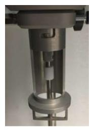
Fill the cup with your product, place it under the measuring head and lower the measuring head to place the centring piece on the cup.
