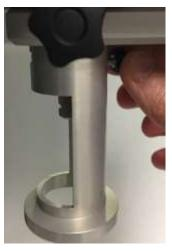
The screw locks the centring piece on the base of the viscometer.
