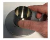
The placement of the centring piece and MK-R2 to MK-R5 is the same as in section 3.9.1. After having installed the centring piece and the MK-Rx spindle, you can lower the measuring head in this position, making sure that the centring piece covers the MB cup.
