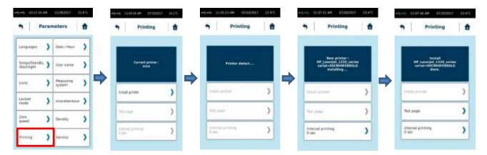
Then you print data at the end of measure or a saved file, you will have only information shown on device screen as final result. If you want to have more data printed, you have to select "Interval printing" time to get data printed between start and end of your measurement.
