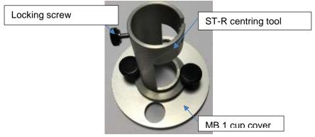
You can install the centring piece and cover assembly on the base of the viscometer. Use the screw to lock the ST-R tool.
