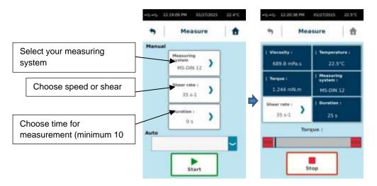
**Rq**: If « Time » = 0, you could modify « speed » <u>during</u> the measurement. This could help you to define the best conditions to work on your sample.
