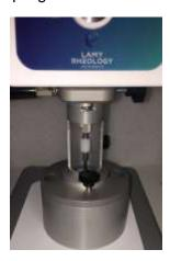
Fill the cup with your product, place under the measuring head and lower the measuring head to place the lid on the cup.
