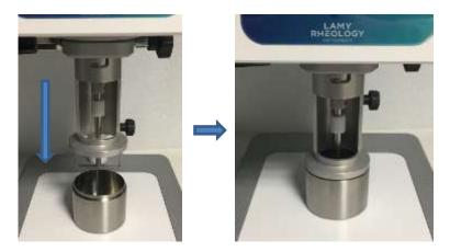
There is no need to block the height of the arm, the viscometer can rest directly on the cup using the centring piece.
