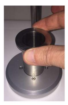
Use the arm handle and screw (see section 1.2) to gently lower the measuring head. The centring piece must completely cover the rim of the tube.
