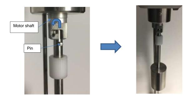
You can then introduce the MS DIN tube with the product from the bottom up slowly and making sure to align with the cylinder. Also place the groove on the tube facing you as shown in the picture below). When you are close enough to the viscometer base, you must rotate the tube to place the pin in the groove of the tube.
