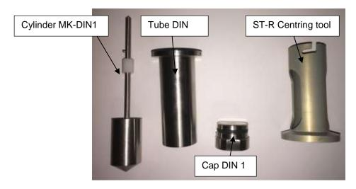
The first step is to install the cap on the tube as shown in the photo below. Also check that the gasket is properly installed on the cap.
