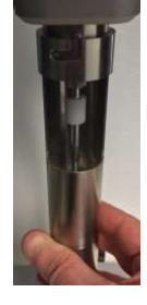
Once the tube is properly installed, check that the temperature sensor on the viscometer is at least one centimetre deep into the liquid.
