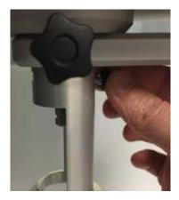
You can then set up the anchor on the bayonet coupling of the viscometer.
