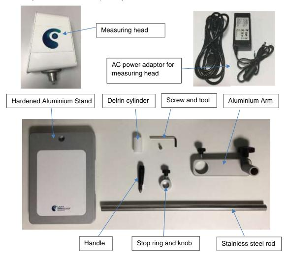
The stop ring is delivered with RM100 PLUS only then MS ASTM or MS KREBS are ordered.
