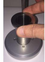
Use handle and screw of arm (see section 1.2) to gently lower the measuring head. The centring piece must completely cover the edge of the disposable cup insert.
