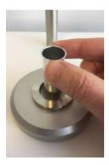
Use handle and screw of arm (see section 1.2) to gently lower the measuring head. The centring piece must completely cover the edge of the disposable cup insert.
