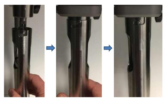
Once the tube is properly installed, check that the temperature sensor on the viscometer is at least one 3mm deep into the liquid.
