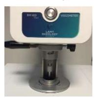
There is no need to block the height of the arm, the viscometer can rest directly on the cup using the centring piece. Also, be sure to allow sufficient time for stabilization if the measurement temperature is different from the ambient temperature (at least 10 minutes) before making your measurement.
